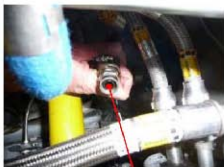
Oil supply hose detail; ID 10,4 mm
