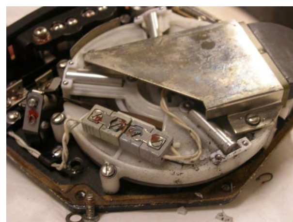
Picture 8: broken tape casing
