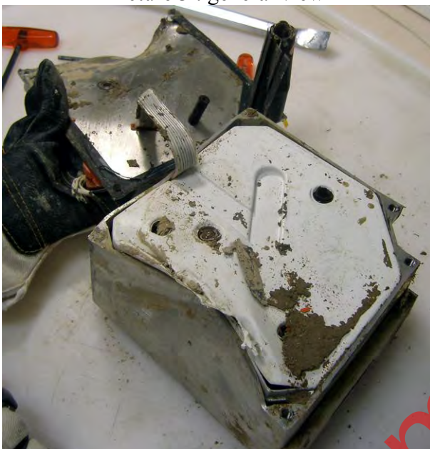
Picture 5 : damaged protected module
